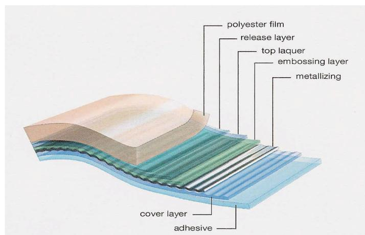
Figure 1 b; a cut away view of an OVD foil
